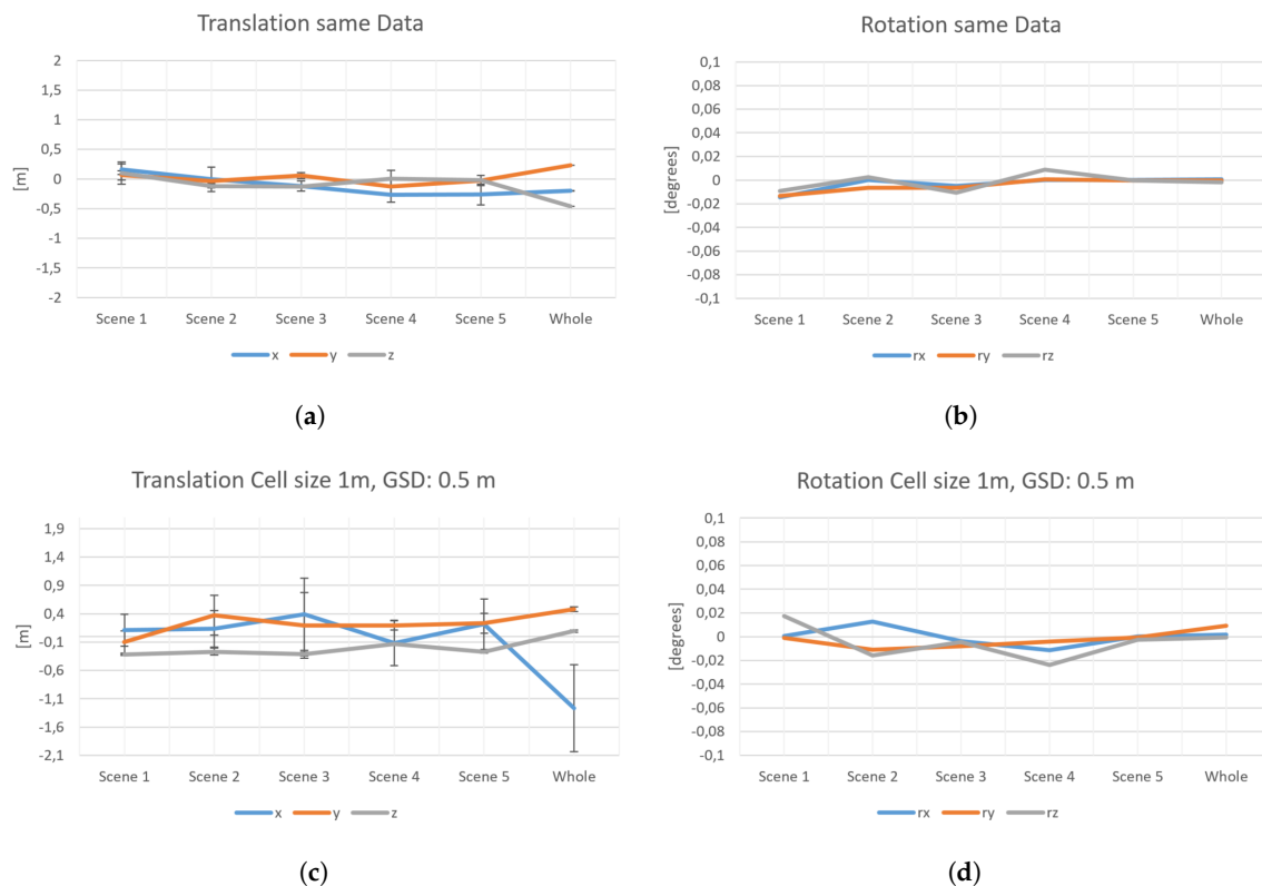
Figure 12. Diagrams of the correctness of calculated transformation parameters. Panels (a) and (b) show the transformation evaluated on the same data with translation parameters (a) and rotation parameters (b). Panels (c) and (d) show the transformation evaluated on the data corresponding to a GSD of 0.5 m with translation parameters (c) and rotation parameters (d). It should be named that there is a change of the grid cell size between the single scenes and the whole data. Single scenes are evaluated using a cell size of about 1 m and the whole data using a cell size of about 4 m.
