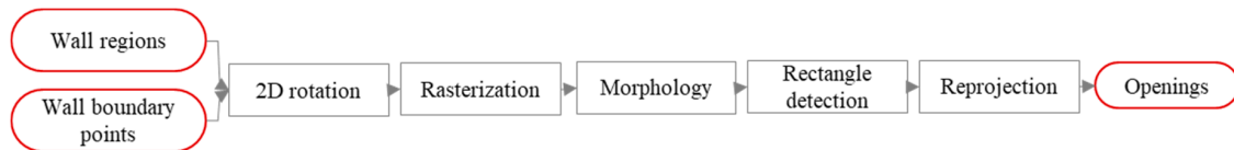
Figure 2. Workflow of the opening detection process.
