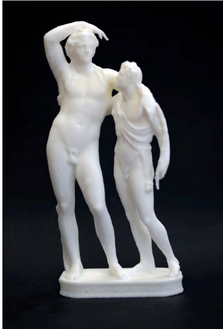
Figure 18. The fused deposition modeling (FDM) replica (a scale of 1:20).
