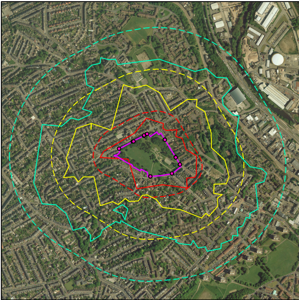
Figure 1. Comparison of areas within network buffers (solid lines) and straight-line buffers (dotted lines) of access points for a greenspace (purple points and boundary), at 100 m (red), 300 m (yellow) and 500 m (blue).
