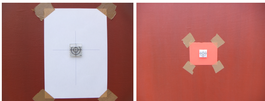
Figure 17. Different targets used in the registration benchmark tests B1 (left) and B2 (right).
