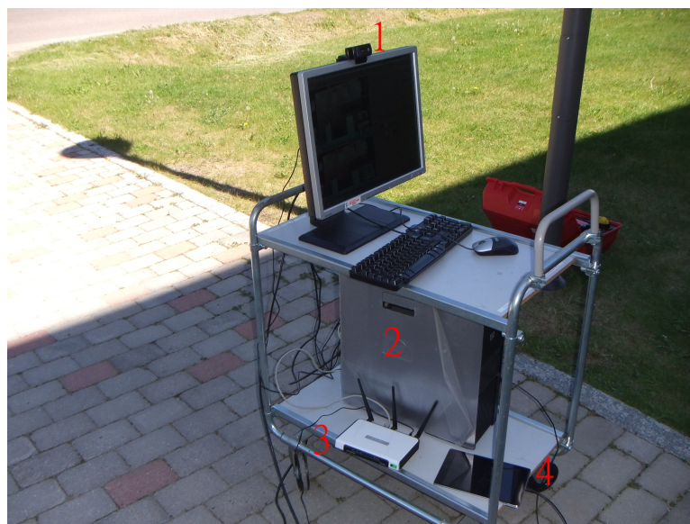
Figure 3. Hardware of the prototype TPP AR system. 1: webcam; 2: desktop computer; 3: wireless router; 4: tablet computer.
