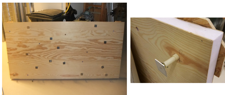
Figure 7. Left: the heating rig with individual heating devices. Right: close-up of a heating device.
