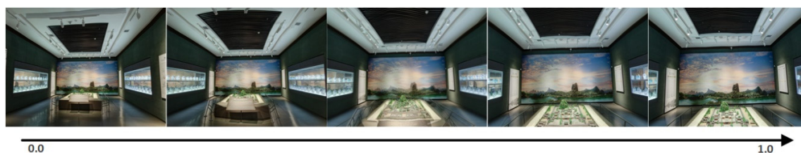
Figure 7. Visual performance of the 360° panoramic walkthrough system with smooth transitions between adjacent viewpoints. The panorama scene transitions from the current site to the next with the process ranging from 0.0 to 1.0.
