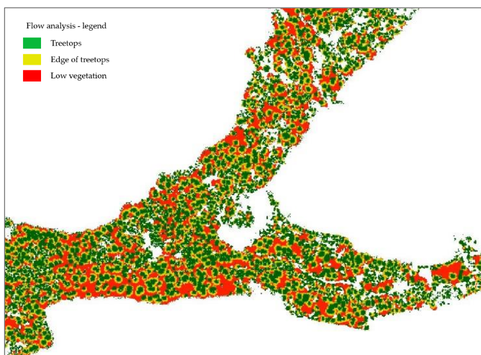
Figure 2. Processing of Digital Surface Model (DSM) based data in the Forest Bačetín with ArcGIS tools Flow analysis, processed and highlighted treetops (green)—the direct method to identify individual trees. Displayed area 600 × 500 m.
