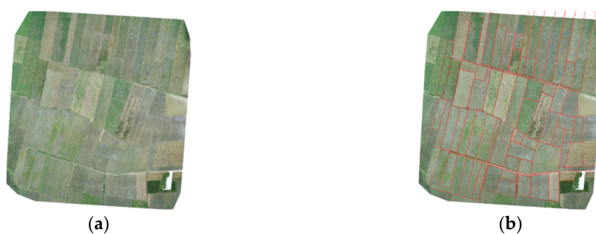
Figure 3. The photos acquired by UAV and the result as the ortho images. (a) The ortho image for one village processed after Pix4D; (b) the image merged with vector data for field blocks.
