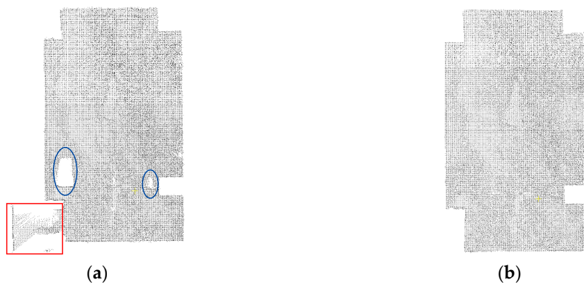
Figure 5. Analysis of the detected floor surface: (a) initial detected floor segment (the points in red rectangle are outliers; the holes in blue ellipses are the occlusions of floor), (b) final floor segment.
