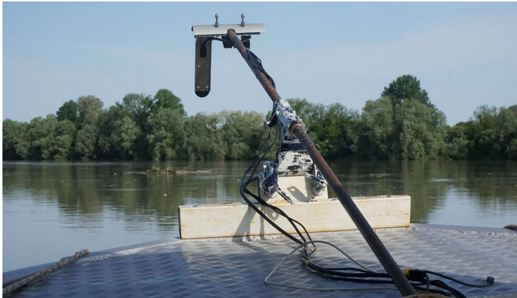
Figure 6. The placement of the sensor array at the bow. The rod can be tilted back to avoid collisions with floating logs. A protective cover is mounted in front of the sensor array to minimize the damage caused by small floating objects.
