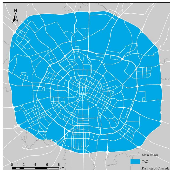
Figure 2. Traffic analysis zones. Traffic analysis zones were obtained by cutting study area with main roads network, and they were taken as the basic spatial unit in this study.
