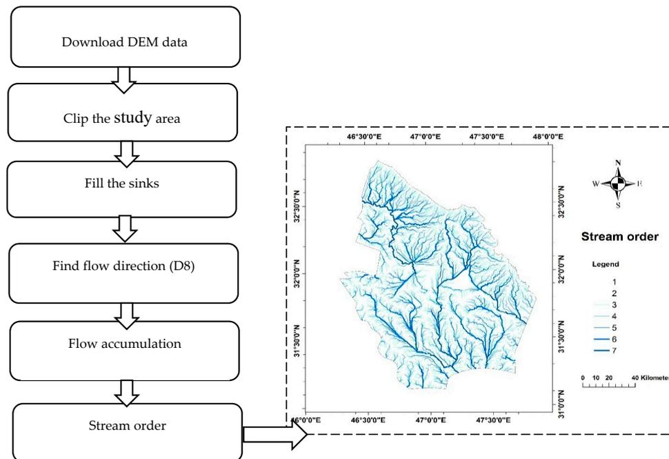
Figure 3. Main steps to derive the stream order based on DEM.
