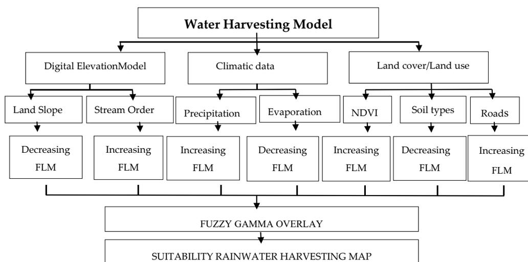
Figure 10. Rainwater harvesting model using Fuzzy Gamma overlay.
