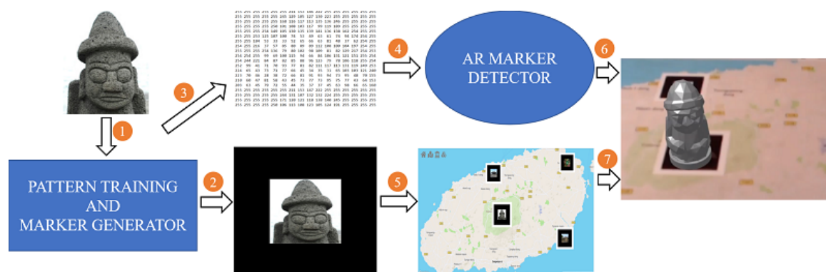
Figure 6. The printed map-making process: (1) representative image of a heritage site, (2) generated marker with augmented region, (3) marker pattern extraction, (4) AR pattern detector, (5) marker inserted into the map, (6) detector marker position, and (7) superimposed artifact on the printed map.
