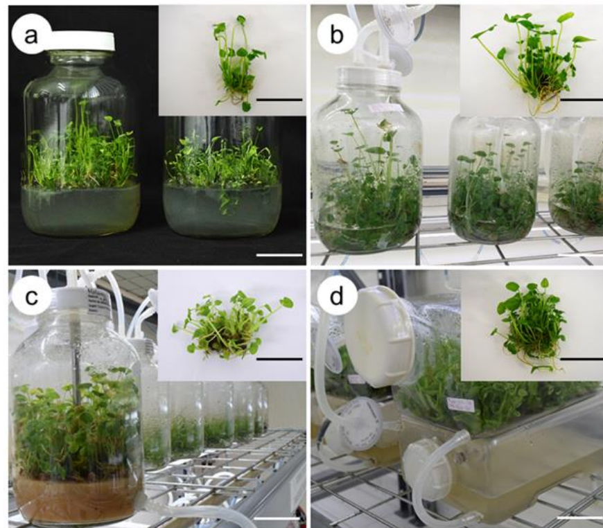
Figure 1. Comparison of culture systems of taro ( Colocasia esculenta ) shoot multiplication after 30 days of culture. (a) Semi-solid medium, (b) temporary immersion bioreactor, (c) ebb-and-flow bioreactor (d) SETIS™ bioreactor. Black and white bar = 5 cm.
