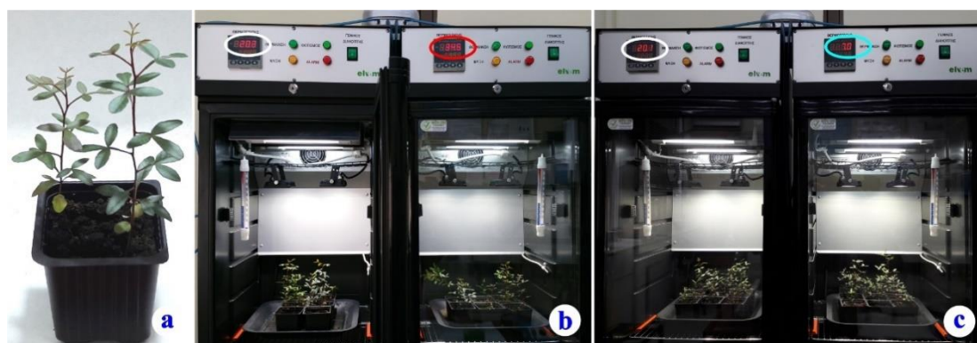
Figure 7. (a). One of the pots with two P. lentiscus plantlets, at the beginning of the experiment. (b) Two of the culture chambers during the heat stress. The control chamber, at the left, and the heat-stress chamber, at the right. Note the temperature reading (34.5 °C) at the moment of the snapshot. (c) Two of the culture chambers during the cold-stress experiment. Note the temperature reading (7.0 °C) at the right chamber.
