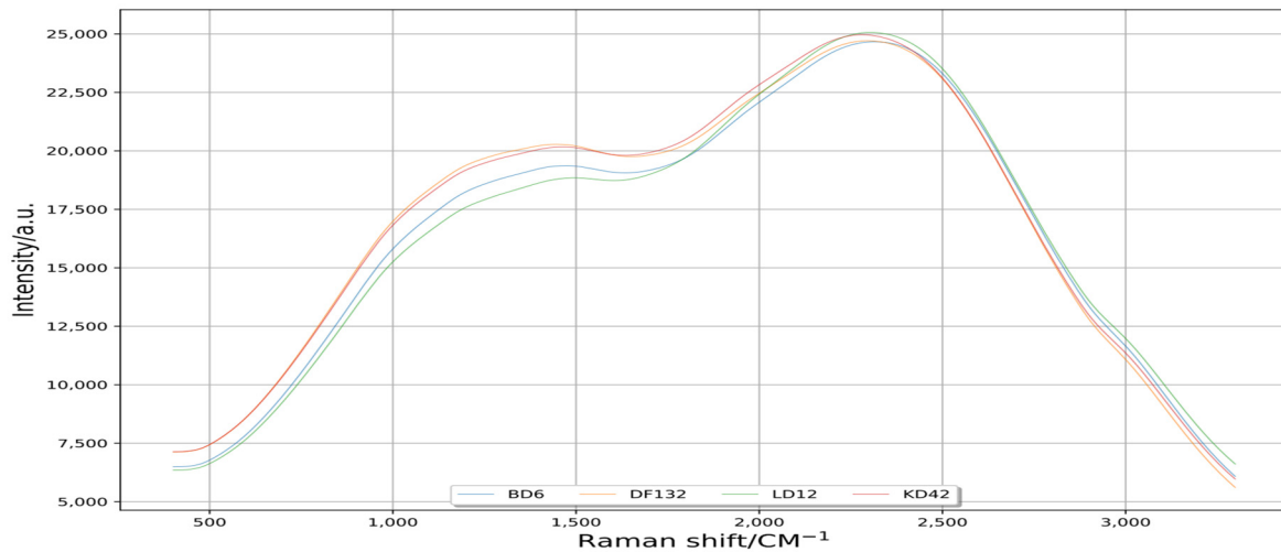
Figure 3. Spectral curves of disturbance reduction by filtering method. Raman shift is the reciprocal of wavelength, unrelated to the frequency of incident light and only related to the vibration frequency of sample molecules, and its range is 200–3400 \text{cm}^{-1} . Intensity is the intensity of Raman scattering, which is the anti-Stokes line; the anti-Stokes line is the scattering light of frequency shifted light from monochromatic incident light in a molecule.
