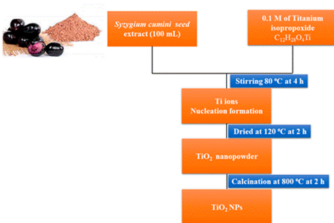
Figure 11. Formation of the TiO 2 NPs from Syzygium cumini seed extract.
