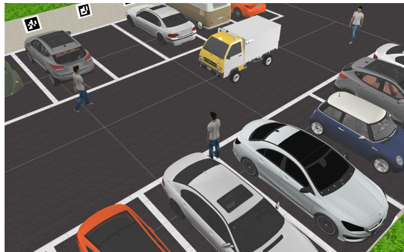
Figure 5. Parking lot scenario developed in ROS and Gazebo Simulator to check the proposed system. The AV is looking for a free parking space in the parking lot and it is navigating among pedestrians and other vehicles depending on the data coming from the perception system and analyzed with the rational agent onboard the AV. The information obtained from the perception system is shown below in Figures 6 and 7.
