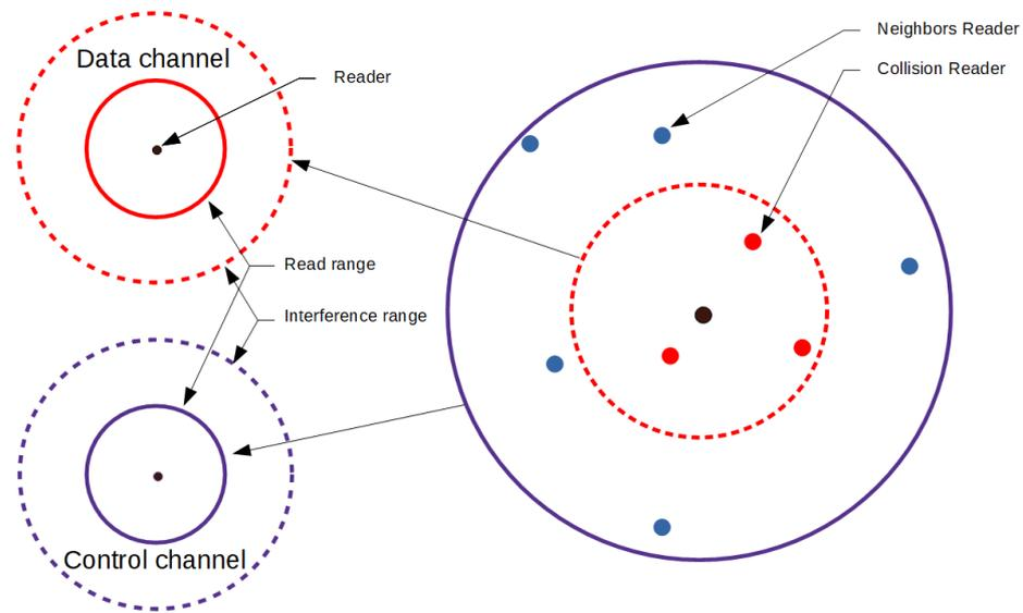
Figure 3. Basic architecture proposed for the RFID reader.
