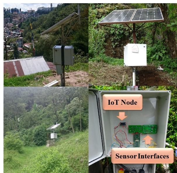
Figure 4. Field nodes (top-left to bottom-right): Node 2 (Tier1), Node 5 (Tier2), Node 10 (Tier3), and their components.
