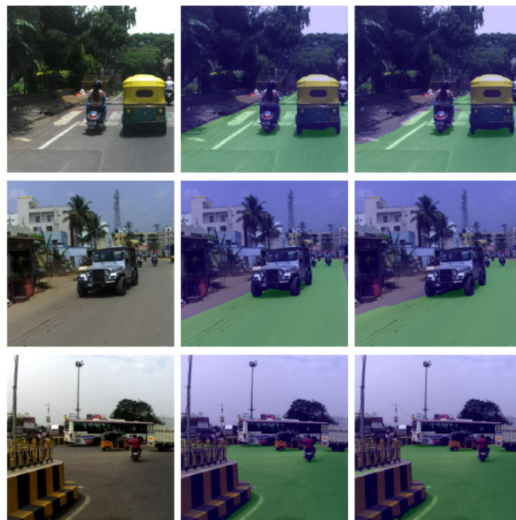
Figure 7. Results of road segmentation on the augmented dataset. The first column shows the input images, while the second and third columns show the ground truth masks and predicted segmentation masks overlapped on the input image, respectively.
