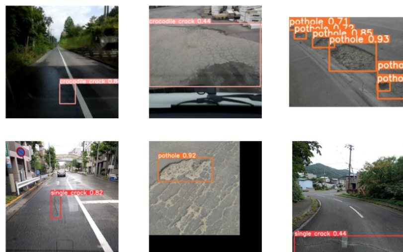
Figure 9. Examples of detection results with the best-performing model: YOLOv5l. It is good to note that the sample at the centre of the bottom row fails to contain an additional bounding box for the visible crocodile crack.
