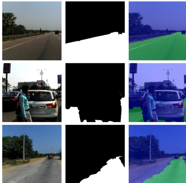
Figure 1. Preprocessed samples of the Indian Driving Dataset (IDD) [4], which depict unstructured urban environments where streets are not well delineated and pedestrians or drivers rarely stick to the rules. The centre and right columns show the ground truth segmentation masks per sample.
