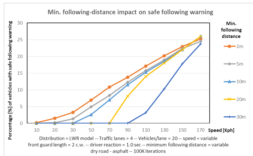
Figure 14. Effect of minimum following distance to safe following warning values at various speeds using LWR traffic distribution.
