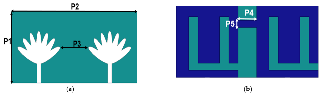
Figure 5. Two-element MIMO configuration: (a) radiator plane; (b) ground plane. Dimensions (in \mu\text{m} ): P1 = 20, P2 = 46, P3 = 6, P4 = 6, P5 = 2.
