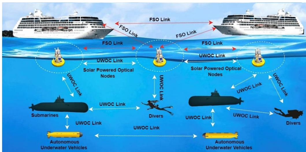
**Figure 1.** Underwater optical wireless communication link.
