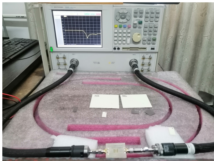
Figure 11. Measurement setup of sensor using Agilent's E8363B Network Analyzer.
