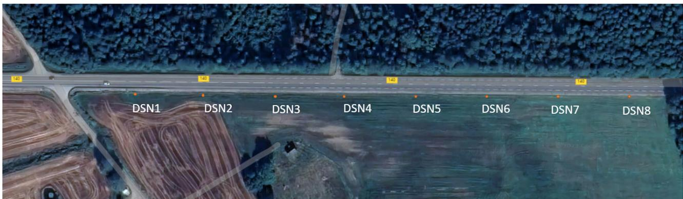
**Figure 3.** Animal detection IoT network with the implemented placement of the DSN nodes.
