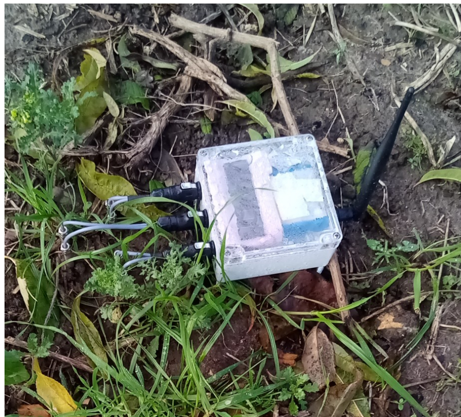
Figure 2. Photo of the new demonstrator operating in the field. The three moisture/salinity probes are visible in the left hand, each sensing a different soil horizon at depths ranging from the surface to 30 cm. The housing contains a Li-ion battery in parallel with a solar cell fixed in the lid. The antenna on the right hand transmits data in real time via LoRaWAN. The thermocouple stick was not used.
