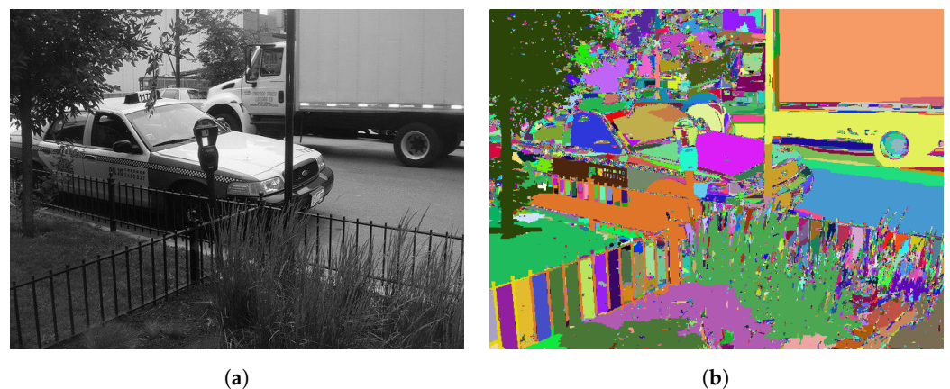
Figure 13. Region segmentation of Taxi: (a) input image, (b) segmented image.
