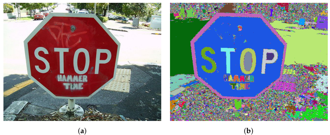
Figure 12. Region segmentation of Stop Sign: (a) input image, (b) segmented image.
