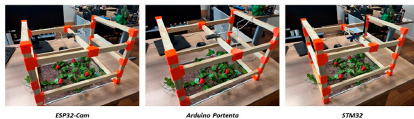
Figure 11. Test bench featuring the ESP32-Cam on the left, the Arduino Portenta in the middle, and the STM32 on the right.
