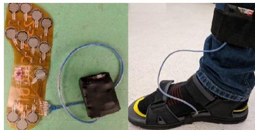
Figure 1. (Left) Flexible PCB with embedded sensors and the control pack containing the WiFi-enabled microcontroller and the 3.3-VLi-ion battery; (Right) a user showing the padded SmartInsole in a sandal while strapping the control pack around the leg.
