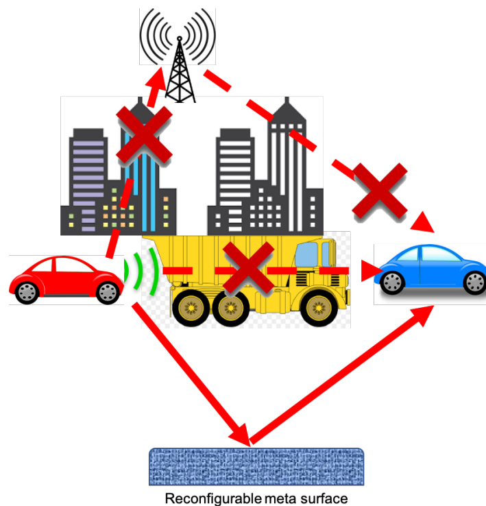
Figure 2. An opportune obstacle coated with meta material to redirect the electromagnetic waves toward the target receiver, which could not be reached through direct link due to an obstacle.
