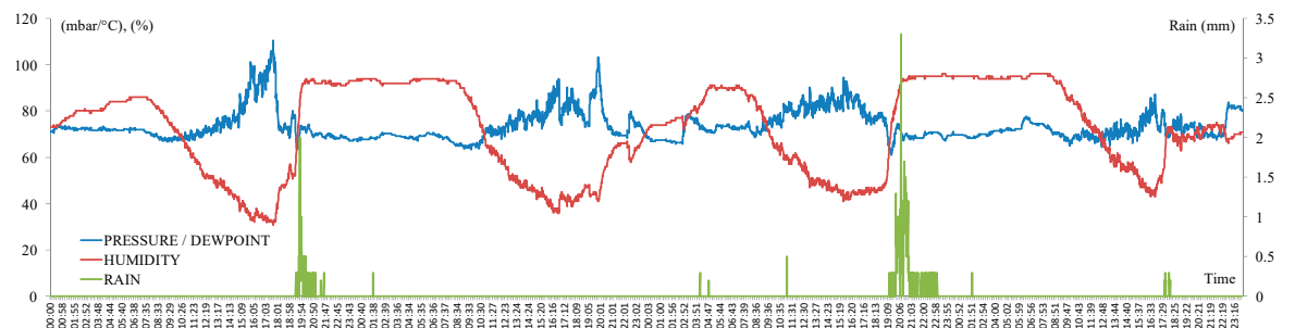
Figure 11. Results of applying the CRHUDA model to UAQ Cerro Campanas data on August 16, 2014 (max depth 55.2 mm in 1 h; max intensity 63.8 mm/h; 53-year return period).
