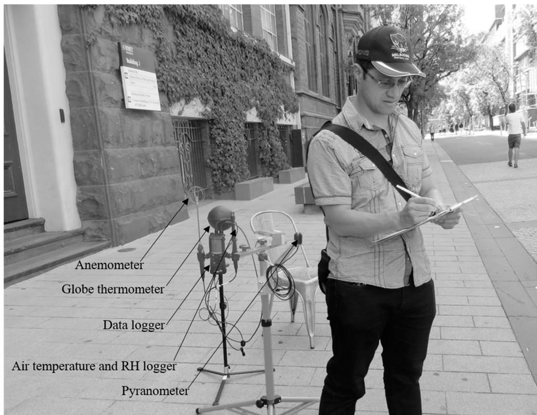
**Figure 4.** Measurement equipment.
