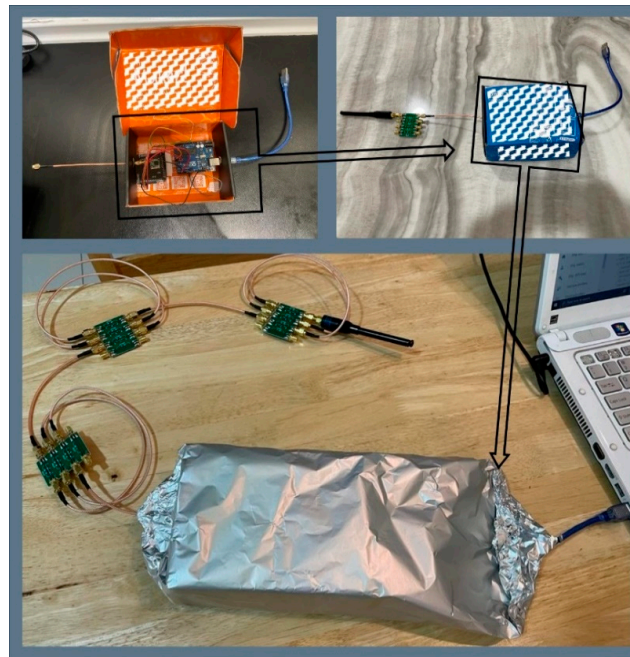
Figure 8. Shielded box to create a Faraday cage-like environment to overcome signal leakage.
