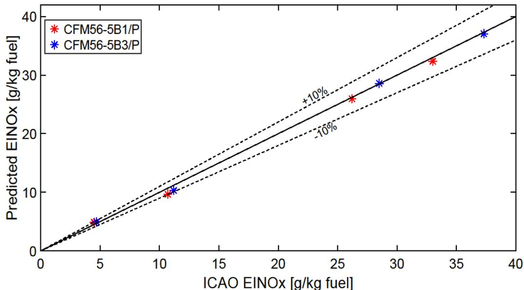
**Figure 4.** Comparison of the model–predicted  $EINO_x$  (Equation (7)) with the ICAO–provided  $EINO_x$  under SLS conditions for two CFM56 models (total eight points) for the rich–burn combustor. The solid dashed line is used as a reference to measure the accuracy of the model, with the dashed lines representing a  $\pm 10\%$  deviation.
