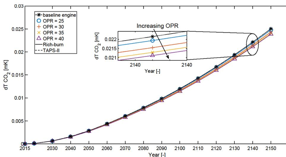
**Figure 18.** Temporal evolution of the temperature response due to CO<sub>2</sub> emissions ( $dT_{CO_2}$ ) for baseline engine (dotted-asterisk line) and the OPR range from 25 to 40. The trends are shown for both combustor technologies (in this case, they result in identical trendlines). The response due to the different configurations is also shown for the year 2140.
