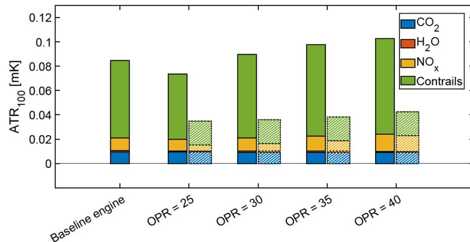
**Figure 23.** Comparison of the  $\text{ATR}_{100}$  for each of the six species for the lowest fuel consumption configurations with changing OPR. The trends for the rich burn combustor are shown in solid, whereas those for the TAPS-II combustor are shown as hatched.
