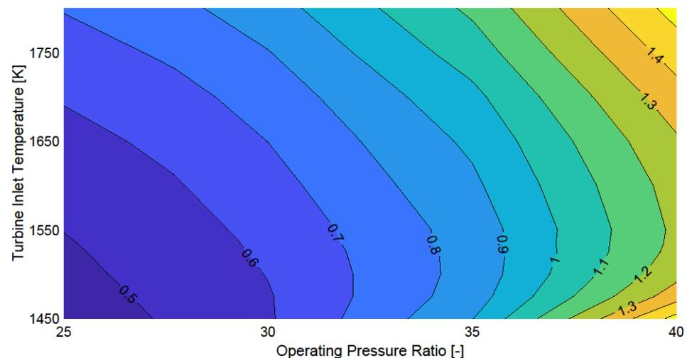
**Figure 15.** Cruise NO<sub>x</sub> emissions of the fleet with varying OPR and TIT for the TAPS-II combustor configurations, normalized to the baseline, which is 3.11 t(NO<sub>2</sub>) (Table 1).
