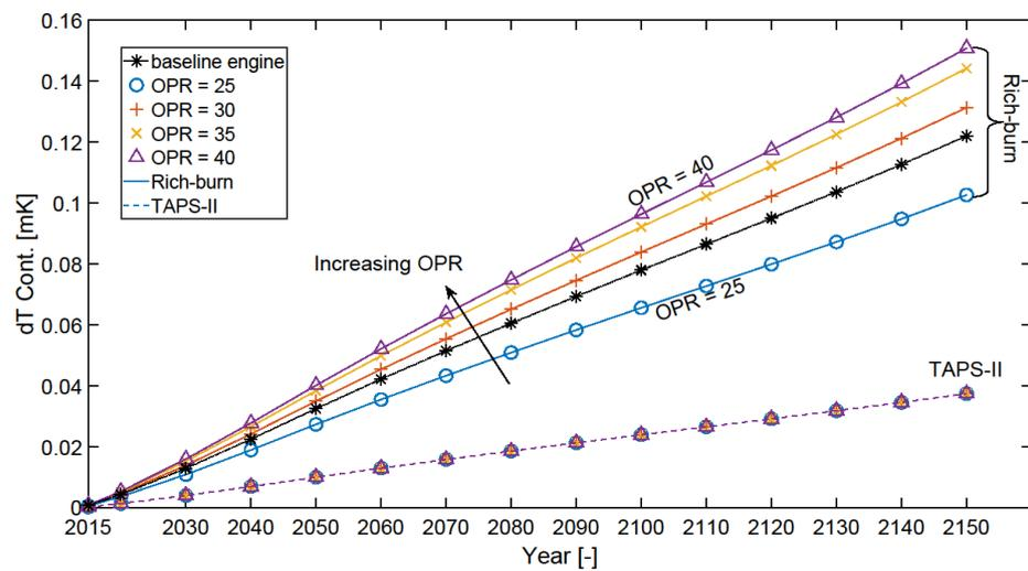
**Figure 20.** Temporal evolution of the temperature response due to contrail effects (dT Cont.) for baseline engine (dotted asterisk line) and the OPR range from 25 to 40. Solid lines represent rich-burn configurations, whereas dashed lines represent TAPS-II configurations.
