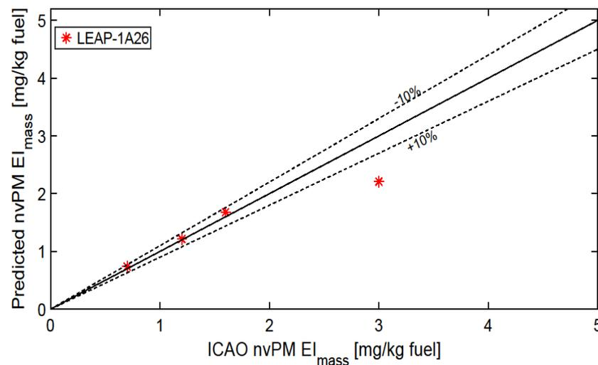
**Figure 7.** Comparison of the model–predicted nvPM  $EI_{mass,SLS}$  (Equation (14)) with ICAO–provided nvPM under SLS conditions for one LEAP–X model (total four points) for the TAPS–II combustor. The solid dashed line is used as a reference to measure the accuracy of the model, with the dashed lines representing a  $\pm 10\%$  deviation.
