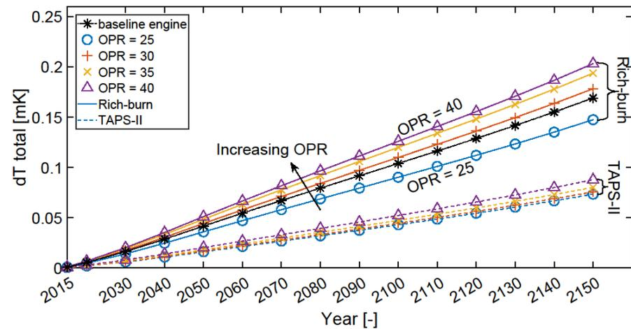
**Figure 22.** Temporal evolution of the total temperature response for baseline engine (dashed asterisk line) and an OPR ranging from 25 to 40. Solid lines represent rich-burn configurations, whereas dashed lines represent TAPS-II configurations.
