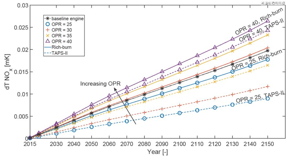
**Figure 19.** Temporal evolution of the temperature response due to NO<sub>x</sub> emissions (enhancement effects due to O<sub>3</sub> production and diminishing effects due to CH<sub>4</sub> and PMO) for baseline engine (dotted asterisk line) and the OPR range from 25 to 40. Solid lines represent rich-burn configurations, whereas dashed lines represent TAPS-II configurations.
