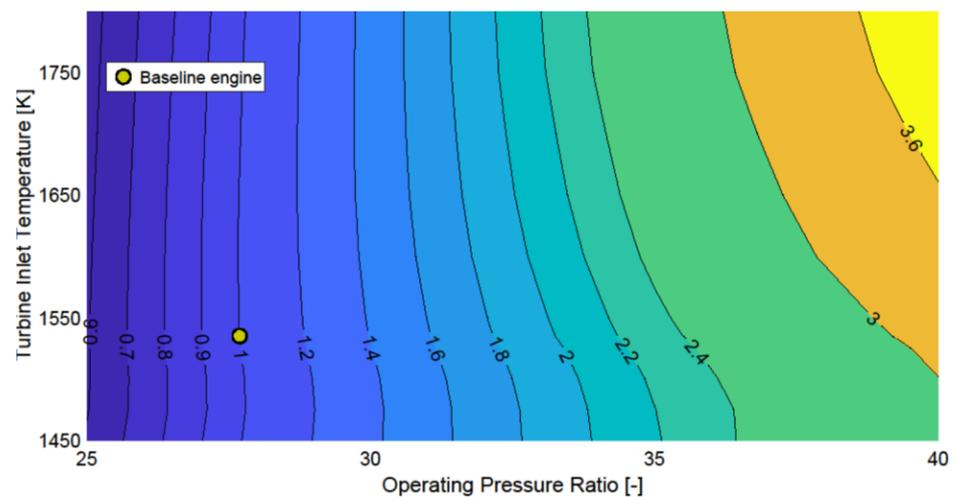
**Figure 13.** Cruise nvPM number of the fleet with varying OPR and TIT for the rich-burn combustor configurations, normalized to the baseline (yellow circle), which is  $1.4 \times 10^{20}$  (#nvPM) (Table 1).
