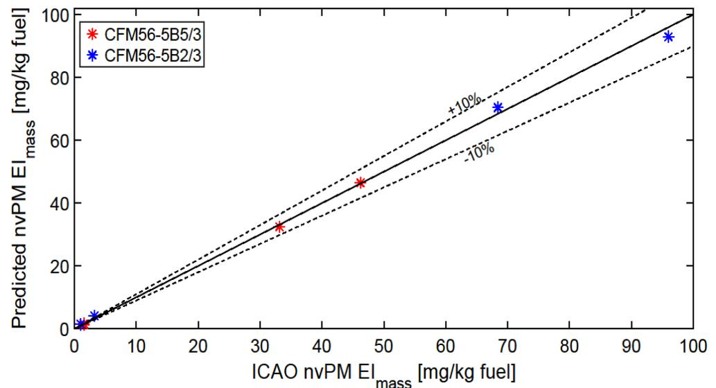
**Figure 5.** Comparison of the model–predicted  $nvPM EI_{mass,SLS}$  (Equation (10)) with ICAO–provided  $nvPM$  under SLS conditions for two CFM56 models (total eight points) for the rich–burn combustor. The solid dashed line is used as a reference to measure the accuracy of the model, with the dashed lines representing a  $\pm 10\%$  deviation.
