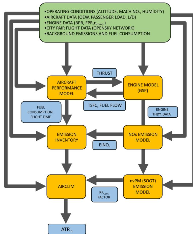
**Figure 2.** The overview of the modeling chain implemented in this research. The contents in green at the top represent the various boundary/operating conditions, those in yellow represent the various models, and those in blue represent the relevant parameters and outputs of interest.
