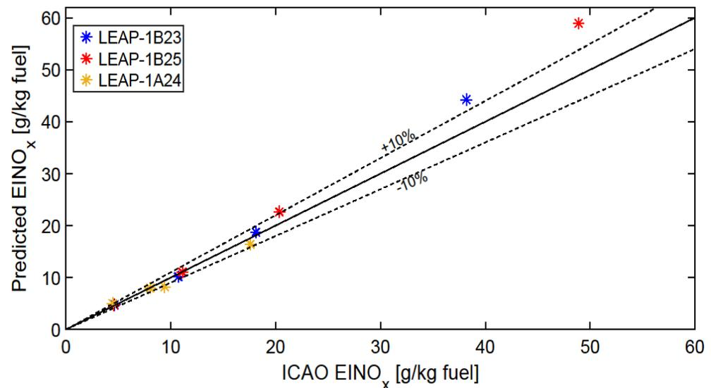
**Figure 6.** Comparison of the model–predicted  $EINO_x$  (Equation (13)) with the ICAO–provided  $EINO_x$  under SLS conditions for three LEAP models (total twelve points) for the TAPS–II combustor. The solid dashed line is used as a reference to measure the accuracy of the model, with the dashed lines representing a  $\pm 10\%$  deviation.
