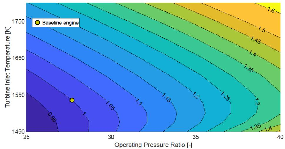
**Figure 12.** Cruise  $\text{NO}_x$  emissions of the fleet with varying OPR and TIT for the rich-burn combustor configurations, normalized to the baseline (yellow circle), which is 3.11 t( $\text{NO}_2$ ) (Table 1).
