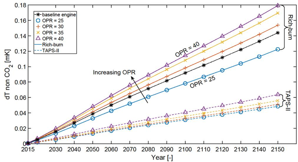
**Figure 21.** Temporal evolution of the temperature response due to the non-CO<sub>2</sub> emissions (dT NO<sub>x</sub>, H<sub>2</sub>O, and contrails) for baseline engine (dotted-asterisk line) and the OPR range from 25 to 40. Solid lines represent rich-burn configurations, whereas dashed lines represent TAPS-II configurations.
