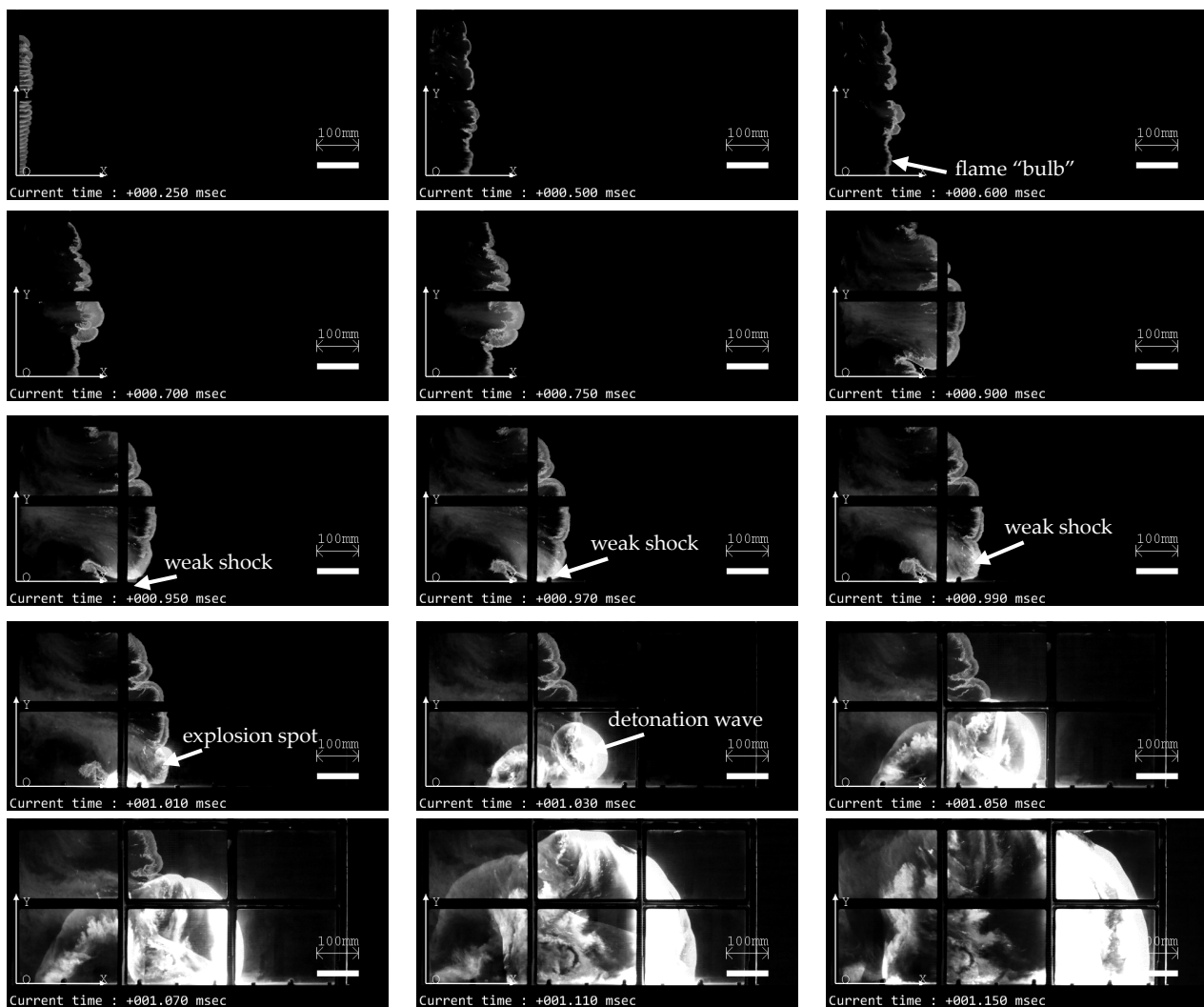
Figure 16. Video frames of flame propagation and DDT in a 1.8\text{C}_2\text{H}_4 + 3\text{O}_2 mixture (experiment no. 545) with h_{\text{est}} = 255 mm: t_{\text{DDT}} = 1.01 ms, X_{\text{DDT}} = 357 mm, Y_{\text{DDT}} = 75 mm.
