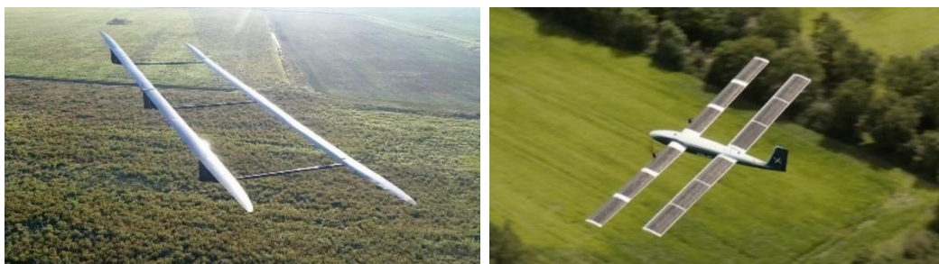
Figure 2. ApusDuo by UAVOS (left) and SolarXOne by XSun (right) tandem-wing prototypes.
