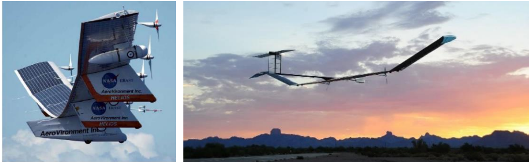
Figure 1. The flying-wing Helios developed by NASA (left) and the wing-tail Airbus Zephyr (right).
