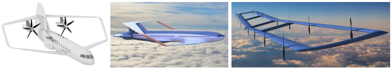
Figure 3. The box-wing architecture applied to regional (left), short-to-medium range (centre) and solar powered (right) aircraft.
