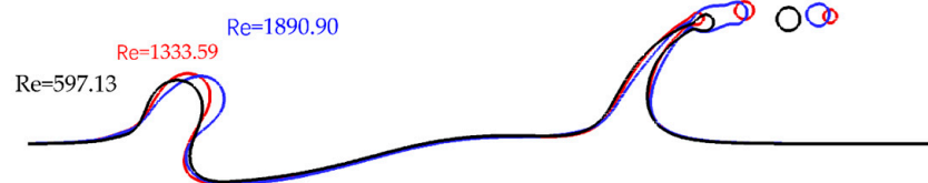
Figure 20. Section of the gas-liquid interfaces with different Reynolds numbers on the Y-mid plane at T = 1.5 .
