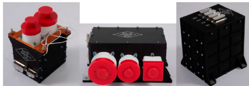
Figure 2. Photos of the high-energy particle detector ((Left panel): -X probe; (central panel): +Y/Z probe; (right panel): electronic box).
