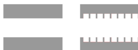
Figure 7. Collimator with smooth inner walls and collimator using collimation structures.
