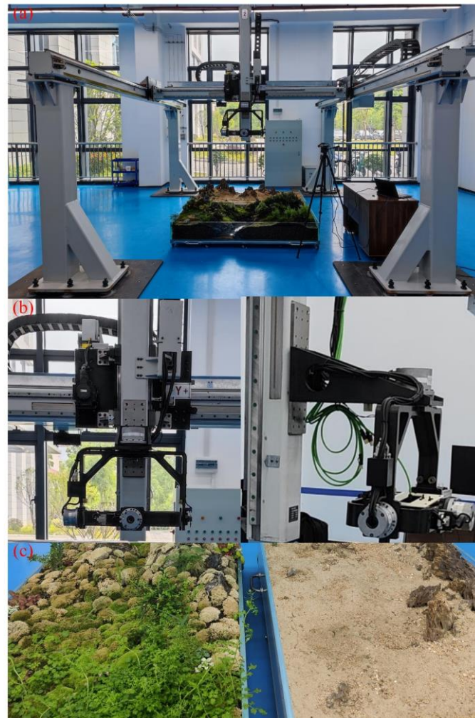
Figure 11. Real system pictures of the simulation system: (a) front view, (b) rotary table, (c) simulation-environment sandbox.
