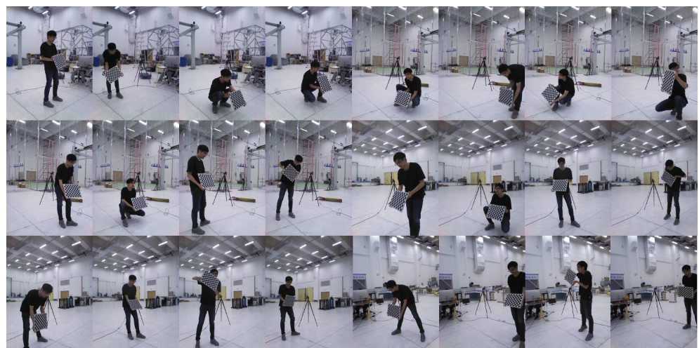
Figure 6. The images samples captured for chessboard calibration. More than 50 pairs of images are captured to guarantee the accuracy of the calibration results.
