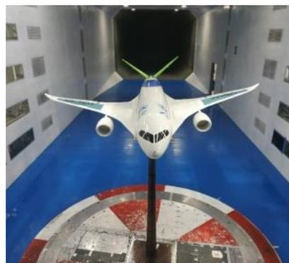
Figure 12. Scaled model in the FL-10 low-speed wind tunnel.
