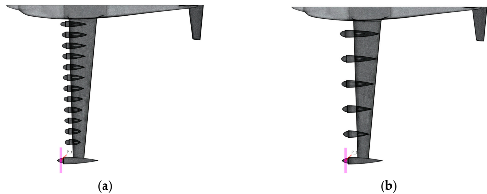
Figure 15. Different configurations of DEP_HP: (a) Cruise configuration with 24 high-lift propellers pylons; (b) Cruise configuration with 10 high-lift propellers pylons.
