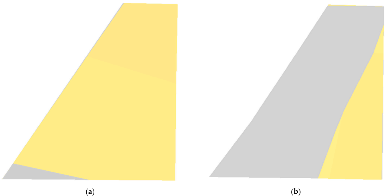
Figure 7. GVT modes of the horizontal tail: (a) the first bending mode; (b) the first torsion mode.
