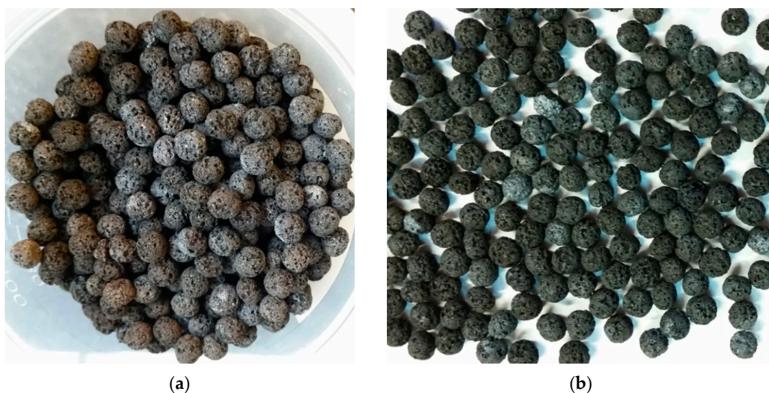
Figure 2. Manganese oxide catalyst, supported on the \alpha -alumina: (a) pre-test view and (b) post-test condition.
