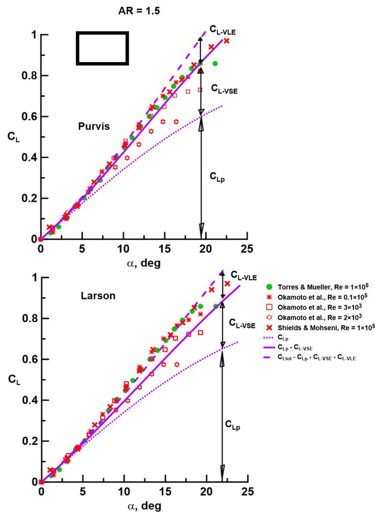
**Figure 4.** Lift coefficient correlation of methods of Purvis and Larson with experimental data for an AR = 1.5 rectangular flat plate wing. Okamoto et al. data from Ref. [2].
