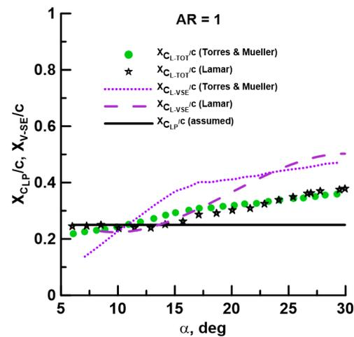
Figure 6. Estimated location of the center of pressure of the attached flow potential lift and side edge vortex lift components, AR = 1.
