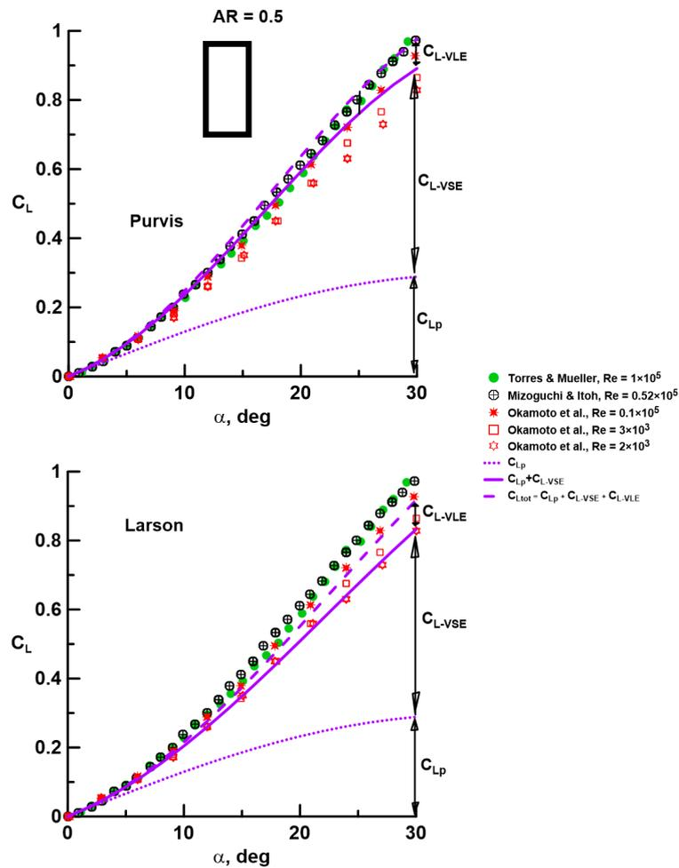
**Figure 2.** Lift coefficient correlation of methods of Purvis and Larson with experimental data for an AR = 0.5 rectangular flat plate wing. Okamoto et al. data from Ref. [2].
