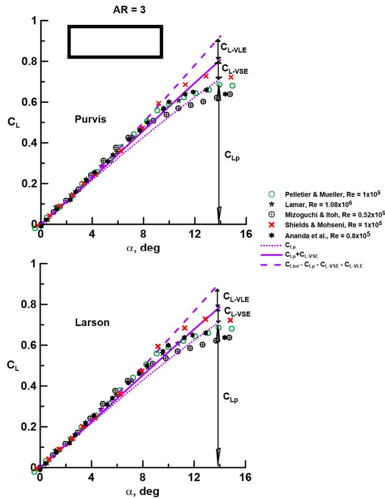
Figure 5. Lift coefficient correlation of methods of Purvis and Larson with experimental data for an AR = 3 rectangular flat plate wing (Ananda et al. data from Ref. [25]).
