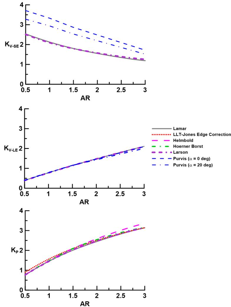
Figure 1. Coefficient estimates for the lift prediction of a rectangular wing.
