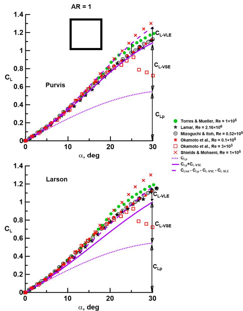
**Figure 3.** Lift coefficient correlation of methods of Purvis and Larson with experimental data for an AR = 1 rectangular flat plate wing. Okamoto et al. data from Ref. [2].
