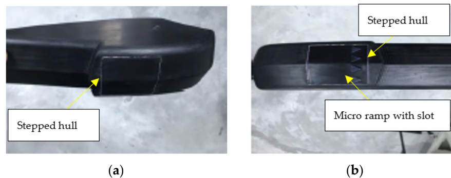
Figure 4. WIG craft fuselage for (a) baseline model (left side) and (b) with micro-ramp (right side).
