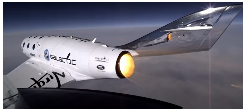
Figure 3. VSS Enterprise fourth rocket powered flight. Note the relatively clean plume of the Nylon-based hybrid rocket motor. From National Transportation Safety Board (NTSB) [107].
