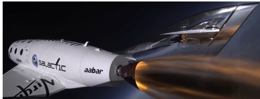
Figure 2. VSS Enterprise third rocket powered flight. Note the relatively smoky plume of the HTPB-based hybrid rocket motor. From Virgin Galactic through The Telegraph [106].
