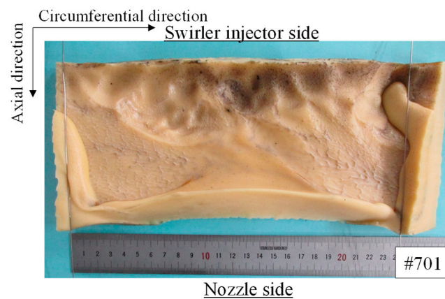
Figure 20. Burned surface of the grain after the test conducted for #701.
