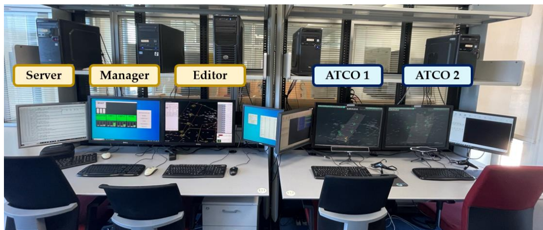
Figure 2. Simulation platform, including the data recording positions (server, manager, and editor) and the simulation positions (ATCO 1 and ATCO 2).
